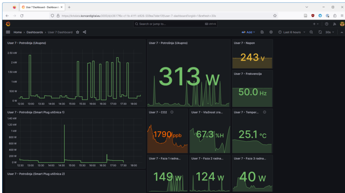
FIGURE 10: [CROATIA DEMO SITE] GRAFANA-BASED DATA COLLECTION PROCESS DEBUG TOOL
