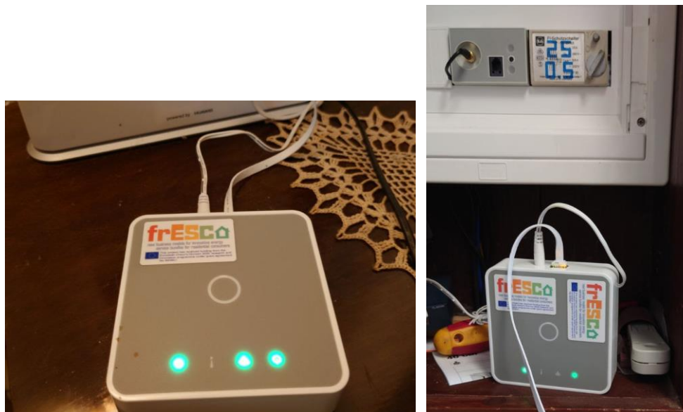
FIGURE 22: [CROATIA DEMO SITE] DEVELCO SQUIDLINK GATEWAYS INSTALLED AND CONFIGURED
