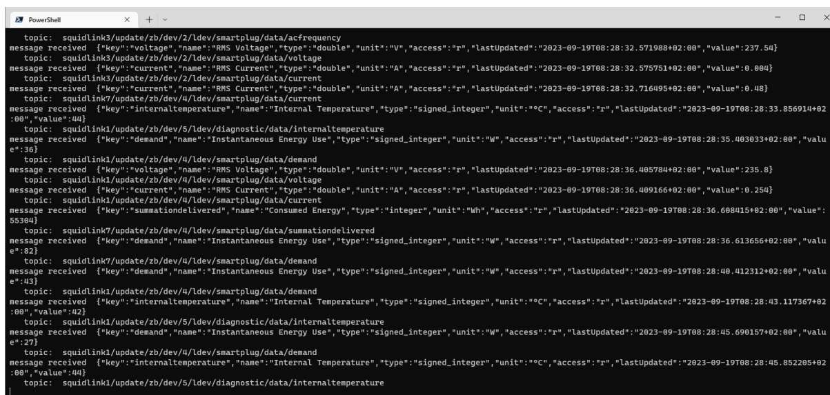
FIGURE 5: [CROATIA DEMO SITE] MQTT CONSUMER COMPONENT INGESTING THE DATA INTO INTERIM DATABASE
